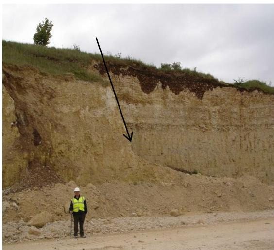
**Figure 5: Normal faulting in the Upper Chalk at Kensworth, arrow indicates fault.**
