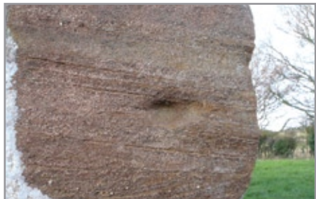
Old St Mary's, Clophill. Note the bedding planes in the sandstone (below), showing how currents shifted the sands on the Cretaceous sea floor.
