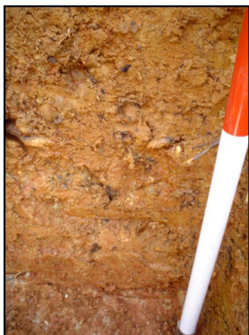
Section showing Reading Formation clays at Downley Common. These clays were present in discontinuous and sinuous outcrops. The result of chasing these thin outcrops is an unnatural landscape full of bumps and hollows.
