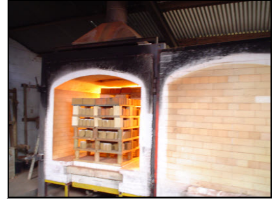
Handmade bricks are being made by H.G. Mathews for specialist purposes. Handmade bricks have a beauty and individuality you cannot obtain with mass production. They are made from the local Reading Formation clays.
