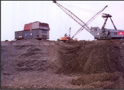
Drag lines operating at Quest Pit before closure, revealing new Oxford Clay exposures.
